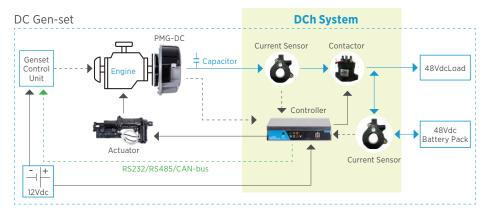
In the event that there is no battery but it is necessary to ensure voltage stability (+/- 1,5%) in all load conditions, a more simplified version can be provided.
